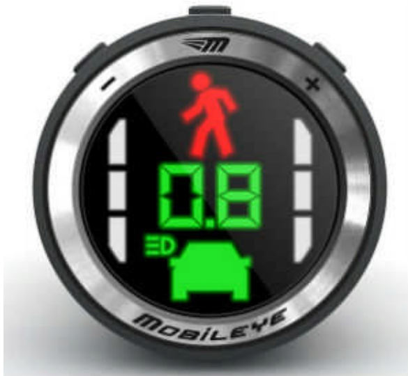
Mobileye shows when a pedestrian is near the vehicle.
